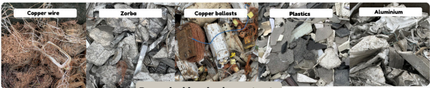
Recycled luminaire outputs
