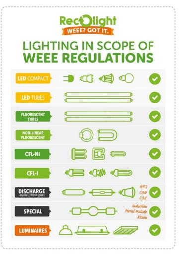
A Luminaire is a complete lighting unit consisting of a lamp or lamps and also the parts which help to position, protect or connect the lamps.
